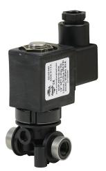
NITRA solenoid valve, 2-way, 2-position, N.C., glass-filled nylon body, 1/8in female NPT inlet(s), 1/8in female NPT outlet(s), Cv=0.12, 24 VAC operating voltage, 18mm DIN style wiring plug.
