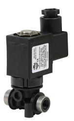
NITRA solenoid valve, 2-way, 2-position, N.C., glass-filled nylon body, 1/8in female NPT inlet(s), 1/8in female NPT outlet(s), Cv=0.12, 120 VAC operating voltage, 18mm DIN style wiring plug.
