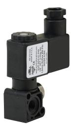
NITRA solenoid valve, 2-way, 2-position, N.C., glass-filled nylon body, 1/8in female NPT inlet(s), 1/8in female NPT outlet(s), stackable, Cv=0.08, 24 VDC operating voltage, 11mm DIN style wiring plug.
