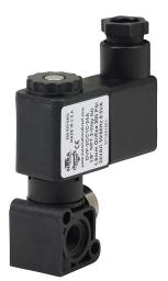
NITRA solenoid valve, 2-way, 2-position, N.C., glass-filled nylon body, 1/8in female NPT inlet(s), 1/8in female NPT outlet(s), stackable, Cv=0.08, 24 VAC operating voltage, 11mm DIN style wiring plug.
