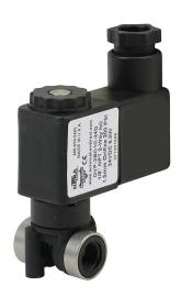
NITRA solenoid valve, 2-way, 2-position, N.C., glass-filled nylon body, 1/8in female NPT inlet(s), 1/8in female NPT outlet(s), Cv=0.08, 24 VDC operating voltage, 11mm DIN style wiring plug.
