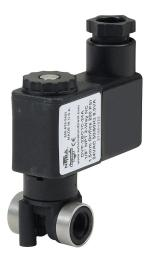
NITRA solenoid valve, 2-way, 2-position, N.C., glass-filled nylon body, 1/8in female NPT inlet(s), 1/8in female NPT outlet(s), Cv=0.08, 24 VAC operating voltage, 11mm DIN style wiring plug.
