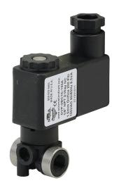
NITRA solenoid valve, 2-way, 2-position, N.C., glass-filled nylon body, 1/8in female NPT inlet(s), 1/8in female NPT outlet(s), Cv=0.08, 120 VAC operating voltage, 11mm DIN style wiring plug.
