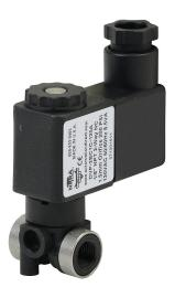
NITRA solenoid valve, 2-way, 2-position, N.C., glass-filled nylon body, 1/8in female NPT inlet(s), 1/8in female NPT outlet(s), Cv=0.08, 120 VAC operating voltage, 11mm DIN style wiring plug.
