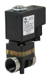
NITRA solenoid valve, 2-way, 2-position, N.C., glass-filled nylon body, 3/8in female NPT inlet(s), 3/8in female NPT outlet(s), Cv=0.52, 24 VDC operating voltage, 18mm DIN style wiring plug.
