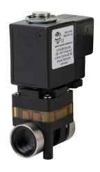
NITRA solenoid valve, 2-way, 2-position, N.C., glass-filled nylon body, 3/8in female NPT inlet(s), 3/8in female NPT outlet(s), Cv=0.52, 24 VAC operating voltage, 18mm DIN style wiring plug.
