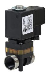
NITRA solenoid valve, 2-way, 2-position, N.C., glass-filled nylon body, 3/8in female NPT inlet(s), 3/8in female NPT outlet(s), Cv=0.52, 120 VAC operating voltage, 18mm DIN style wiring plug.
