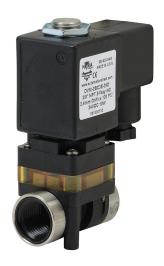
NITRA solenoid valve, 2-way, 2-position, N.C., glass-filled nylon body, 3/8in female NPT inlet(s), 3/8in female NPT outlet(s), Cv=0.24, 24 VDC operating voltage, 18mm DIN style wiring plug.
