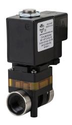
NITRA solenoid valve, 2-way, 2-position, N.C., glass-filled nylon body, 3/8in female NPT inlet(s), 3/8in female NPT outlet(s), Cv=0.24, 24 VAC operating voltage, 18mm DIN style wiring plug.
