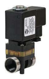
NITRA solenoid valve, 2-way, 2-position, N.C., glass-filled nylon body, 3/8in female NPT inlet(s), 3/8in female NPT outlet(s), Cv=0.24, 120 VAC operating voltage, 18mm DIN style wiring plug.
