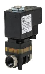
NITRA solenoid valve, 2-way, 2-position, N.C., glass-filled nylon body, 1/4in female NPT inlet(s), 1/4in female NPT outlet(s), Cv=0.52, 24 VDC operating voltage, 18mm DIN style wiring plug.
