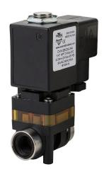
NITRA solenoid valve, 2-way, 2-position, N.C., glass-filled nylon body, 1/4in female NPT inlet(s), 1/4in female NPT outlet(s), Cv=0.52, 24 VAC operating voltage, 18mm DIN style wiring plug.
