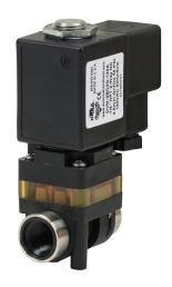
NITRA solenoid valve, 2-way, 2-position, N.C., glass-filled nylon body, 1/4in female NPT inlet(s), 1/4in female NPT outlet(s), Cv=0.52, 120 VAC operating voltage, 18mm DIN style wiring plug.
