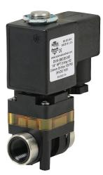
NITRA solenoid valve, 2-way, 2-position, N.C., glass-filled nylon body, 1/4in female NPT inlet(s), 1/4in female NPT outlet(s), Cv=0.24, 24 VDC operating voltage, 18mm DIN style wiring plug.
