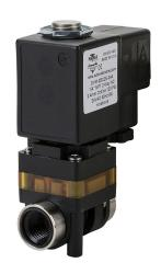
NITRA solenoid valve, 2-way, 2-position, N.C., glass-filled nylon body, 1/4in female NPT inlet(s), 1/4in female NPT outlet(s), Cv=0.24, 24 VAC operating voltage, 18mm DIN style wiring plug.
