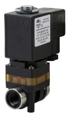
NITRA solenoid valve, 2-way, 2-position, N.C., glass-filled nylon body, 1/4in female NPT inlet(s), 1/4in female NPT outlet(s), Cv=0.24, 120 VAC operating voltage, 18mm DIN style wiring plug.
