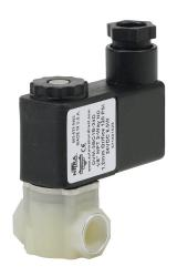
NITRA solenoid valve, 2-way, 2-position, N.C., glass-filled nylon body, 1/8in female NPT inlet(s), 1/8in female NPT outlet(s), Cv=0.065, 24 VDC operating voltage, 11mm DIN style wiring plug.
