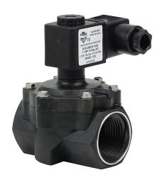
NITRA solenoid valve, 2-way, 2-position, N.C., brass and composite body, 1in female NPT inlet(s), 1in female NPT outlet(s), Cv=14, 24 VDC operating voltage, 18mm DIN style wiring plug.
