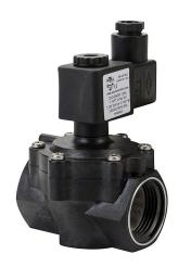
NITRA solenoid valve, 2-way, 2-position, N.C., brass and composite body, 1in female NPT inlet(s), 1in female NPT outlet(s), Cv=14, 120 VAC operating voltage, 18mm DIN style wiring plug.
