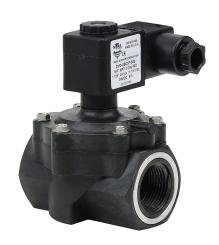
NITRA solenoid valve, 2-way, 2-position, N.C., brass and composite body, 3/4in female NPT inlet(s), 3/4in female NPT outlet(s), Cv=14, 24 VDC operating voltage, 18mm DIN style wiring plug.
