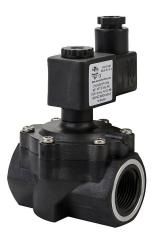
NITRA solenoid valve, 2-way, 2-position, N.C., brass and composite body, 3/4in female NPT inlet(s), 3/4in female NPT outlet(s), Cv=14, 120 VAC operating voltage, 18mm DIN style wiring plug.
