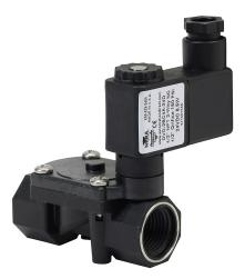
NITRA solenoid valve, 2-way, 2-position, N.C., glass-filled nylon body, 1/2in female NPT inlet(s), 1/2in female NPT outlet(s), Cv=2.45, 24 VDC operating voltage, 11mm DIN style wiring plug.
