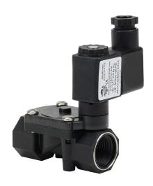
NITRA solenoid valve, 2-way, 2-position, N.C., glass-filled nylon body, 1/2in female NPT inlet(s), 1/2in female NPT outlet(s), Cv=2.45, 24 VAC operating voltage, 11mm DIN style wiring plug.
