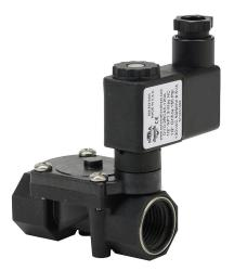
NITRA solenoid valve, 2-way, 2-position, N.C., glass-filled nylon body, 1/2in female NPT inlet(s), 1/2in female NPT outlet(s), Cv=2.45, 120 VAC operating voltage, 11mm DIN style wiring plug.
