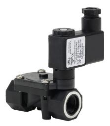
NITRA solenoid valve, 2-way, 2-position, N.C., glass-filled nylon body, 3/8in female NPT inlet(s), 3/8in female NPT outlet(s), Cv=1.95, 24 VDC operating voltage, 11mm DIN style wiring plug.
