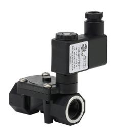
NITRA solenoid valve, 2-way, 2-position, N.C., glass-filled nylon body, 3/8in female NPT inlet(s), 3/8in female NPT outlet(s), Cv=1.95, 24 VAC operating voltage, 11mm DIN style wiring plug.
