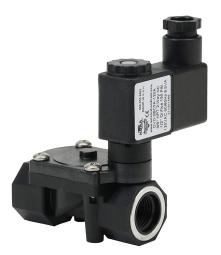
NITRA solenoid valve, 2-way, 2-position, N.C., glass-filled nylon body, 3/8in female NPT inlet(s), 3/8in female NPT outlet(s), Cv=1.95, 120 VAC operating voltage, 11mm DIN style wiring plug.
