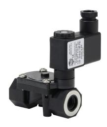
NITRA solenoid valve, 2-way, 2-position, N.C., glass-filled nylon body, 1/4in female NPT inlet(s), 1/4in female NPT outlet(s), Cv=1.55, 24 VDC operating voltage, 11mm DIN style wiring plug.
