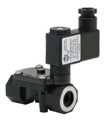
NITRA solenoid valve, 2-way, 2-position, N.C., glass-filled nylon body, 1/4in female NPT inlet(s), 1/4in female NPT outlet(s), Cv=1.55, 120 VAC operating voltage, 11mm DIN style wiring plug.
