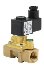
NITRA solenoid valve, 2-way, 2-position, N.C., brass body, 1/2in female NPT inlet(s), 1/2in female NPT outlet(s), Cv=2.45, 24 VDC operating voltage, 18mm DIN style wiring plug.
