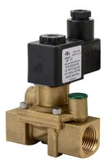
NITRA solenoid valve, 2-way, 2-position, N.C., brass body, 1/2in female NPT inlet(s), 1/2in female NPT outlet(s), Cv=2.45, 24 VAC operating voltage, 18mm DIN style wiring plug.
