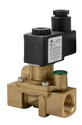
NITRA solenoid valve, 2-way, 2-position, N.C., brass body, 1/2in female NPT inlet(s), 1/2in female NPT outlet(s), Cv=2.45, 120 VAC operating voltage, 18mm DIN style wiring plug.
