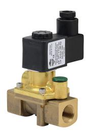
NITRA solenoid valve, 2-way, 2-position, N.C., brass body, 3/8in female NPT inlet(s), 3/8in female NPT outlet(s), Cv=1.95, 24 VDC operating voltage, 18mm DIN style wiring plug.
