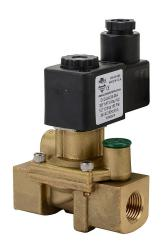
NITRA solenoid valve, 2-way, 2-position, N.C., brass body, 3/8in female NPT inlet(s), 3/8in female NPT outlet(s), Cv=1.95, 24 VAC operating voltage, 18mm DIN style wiring plug.
