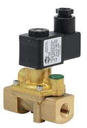
NITRA solenoid valve, 2-way, 2-position, N.C., brass body, 1/4in female NPT inlet(s), 1/4in female NPT outlet(s), Cv=1.55, 24 VDC operating voltage, 18mm DIN style wiring plug.
