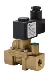
NITRA solenoid valve, 2-way, 2-position, N.C., brass body, 1/4in female NPT inlet(s), 1/4in female NPT outlet(s), Cv=1.55, 24 VAC operating voltage, 18mm DIN style wiring plug.
