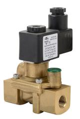
NITRA solenoid valve, 2-way, 2-position, N.C., brass body, 1/4in female NPT inlet(s), 1/4in female NPT outlet(s), Cv=1.55, 120 VAC operating voltage, 18mm DIN style wiring plug.
