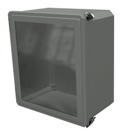
Stahlin Diamond Shield series enclosure, NEMA 1/3/3S/4X/12/13,  $18 \times 16 \times 10$  in (HxWxD), wall mount, fiberglass reinforced polyester, gray, crowned single-door, (2) quick-release latches, padlock hasp and staple, SAR acrylic window.
