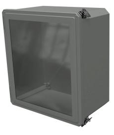
Stahlin Diamond Shield series enclosure, NEMA 1/3/3S/4X/12/13, 18 x 16 x 10in (HxWxD), wall mount, fiberglass reinforced polyester, gray, crowned single-door, (2) twist-lock latches, padlock hasp and staple, SAR acrylic window.
