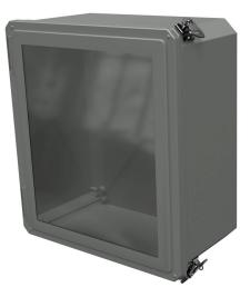
Stahlin Diamond Shield series enclosure, NEMA 1/3/3S/4X/12/13, 16 x 14 x 8in (HxWxD), wall mount, fiberglass reinforced polyester, gray, crowned single-door, (2) twist-lock latches, padlock hasp and staple, SAR acrylic window.
