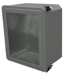
Stahlin Diamond Shield series enclosure, NEMA 1/3/3S/4X/12/13, 14 x 12 x 8in (HxWxD), wall mount, fiberglass reinforced polyester, gray, crowned single-door, (2) quick-release latches, padlock hasp and staple, SAR acrylic window.
