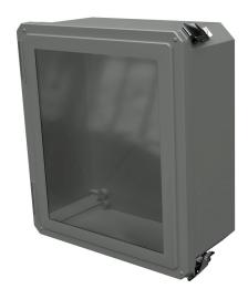
Stahlin Diamond Shield series enclosure, NEMA 1/3/3S/4X/12/13, 14 x 12 x 6in (HxWxD), wall mount, fiberglass reinforced polyester, gray, crowned single-door, (2) quick-release latches, padlock hasp and staple, SAR acrylic window.
