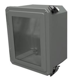
Stahlin Diamond Shield series enclosure, NEMA 1/3/3S/4X/12/13,  $10 \times 8 \times 6$  in (HxWxD), wall mount, fiberglass reinforced polyester, gray, crowned single-door, (2) quick-release latches, padlock hasp and staple, SAR acrylic window.
