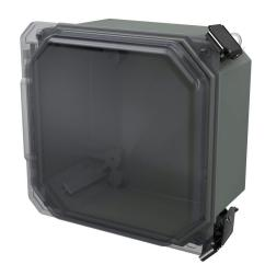
Stahlin Diamond Shield series enclosure, NEMA 1/3/3S/4X/12/13, 6 x 6 x 4in (HxWxD), wall mount, fiberglass reinforced polyester, gray, clear polycarbonate single-door, (2) quick-release latches, padlock hasp and staple.
