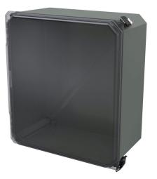
Stahlin Diamond Shield series enclosure, NEMA 1/3/3S/4X/12/13, 16 x 14 x 8in (HxWxD), wall mount, fiberglass reinforced polyester, gray, clear polycarbonate single-door, (2) quick-release latches, padlock hasp and staple.
