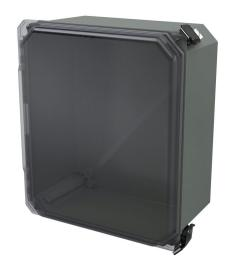
Stahlin Diamond Shield series enclosure, NEMA 1/3/3S/4X/12/13,  $12 \times 10 \times 6$  in (HxWxD), wall mount, fiberglass reinforced polyester, gray, clear polycarbonate single-door, (2) quick-release latches, padlock hasp and staple.
