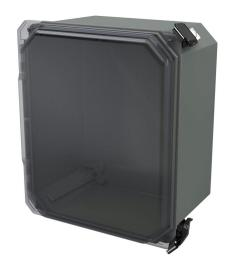
Stahlin Diamond Shield series enclosure, NEMA 1/3/3S/4X/12/13,  $10 \times 8 \times 6$  in (HxWxD), wall mount, fiberglass reinforced polyester, gray, clear polycarbonate single-door, (2) quick-release latches, padlock hasp and staple.
